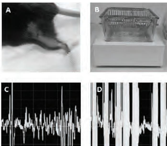
Software-based method to record scratch activity. A) Teflon-coated magnets implanted in both hind paws induce electric currents through B) magnetic coils around cages. C/D) Software can distinguish between body movement (C) and scratching (D).
